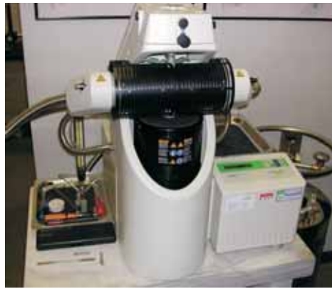
Figure 5—The Dynamic Mechanical Analysis (DMA), used for measuring Tg.
