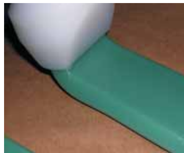
Close-up of extruded bead of tooling paste as dispensed.
