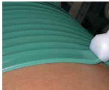
Paste being applied onto male mold shape with dispensing equipment.
