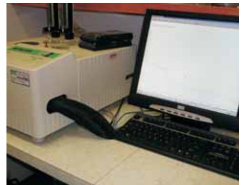
Figure 2—The Differential Scanning Calorimeter (DSC), used to measure Tg.
