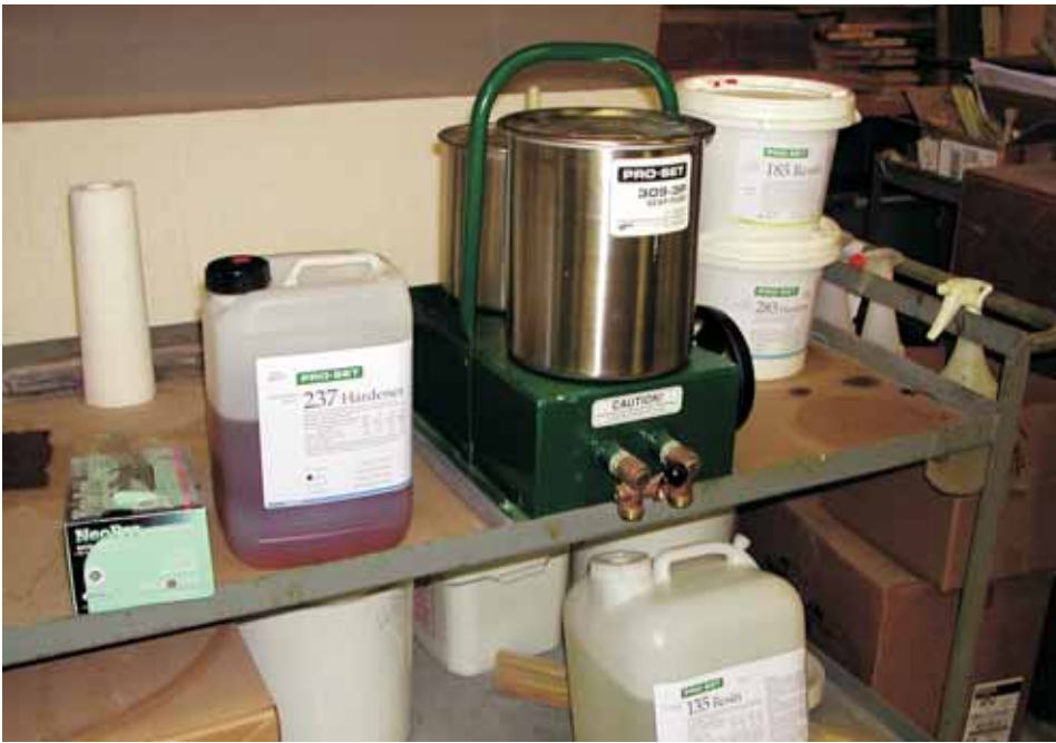
Typical 309-P Gear Pump station. Check the ratio daily.
