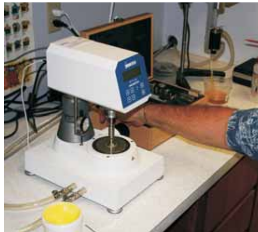
The rotating element is lowered onto a small amount of filled resin on the measuring plate.
