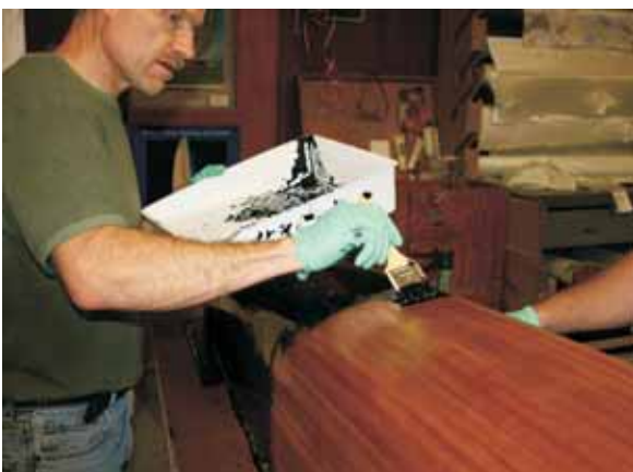
Tom Pawlak applies M1019 black surface coat resin with 224 (fast) hardener to the waxed, wooden plug.
