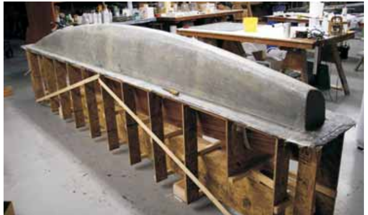
The first half-mold for the starboard side of the decked canoe is laid up, ready for a framework and lay up of the port half-mold.
