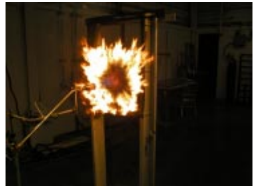
PRO-SET laminate sample during 2900° F flame testing at Underwriter’s Laboratories
