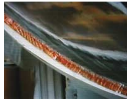
Cut-away of the hull showing excess fairing.
